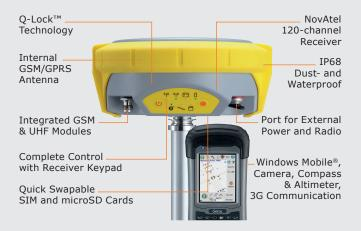
The Q-Lock™ technology tracks all satellites with the highest available signal strength and performs regular independent checks to ensure that you can work even in challenging environments such as urban canyons or under heavy foliage.
